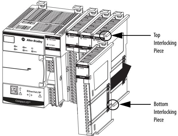
7. Verify that the module is installed in one of the following ways:
