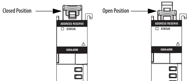
5. Align the interlocking pieces of the module with the device on the left. The top interlocking pieces engage first.
